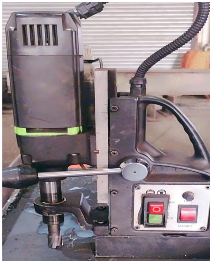
PORTABLE DRILLING MACHINES (Capacity-Dia-60 mm)
