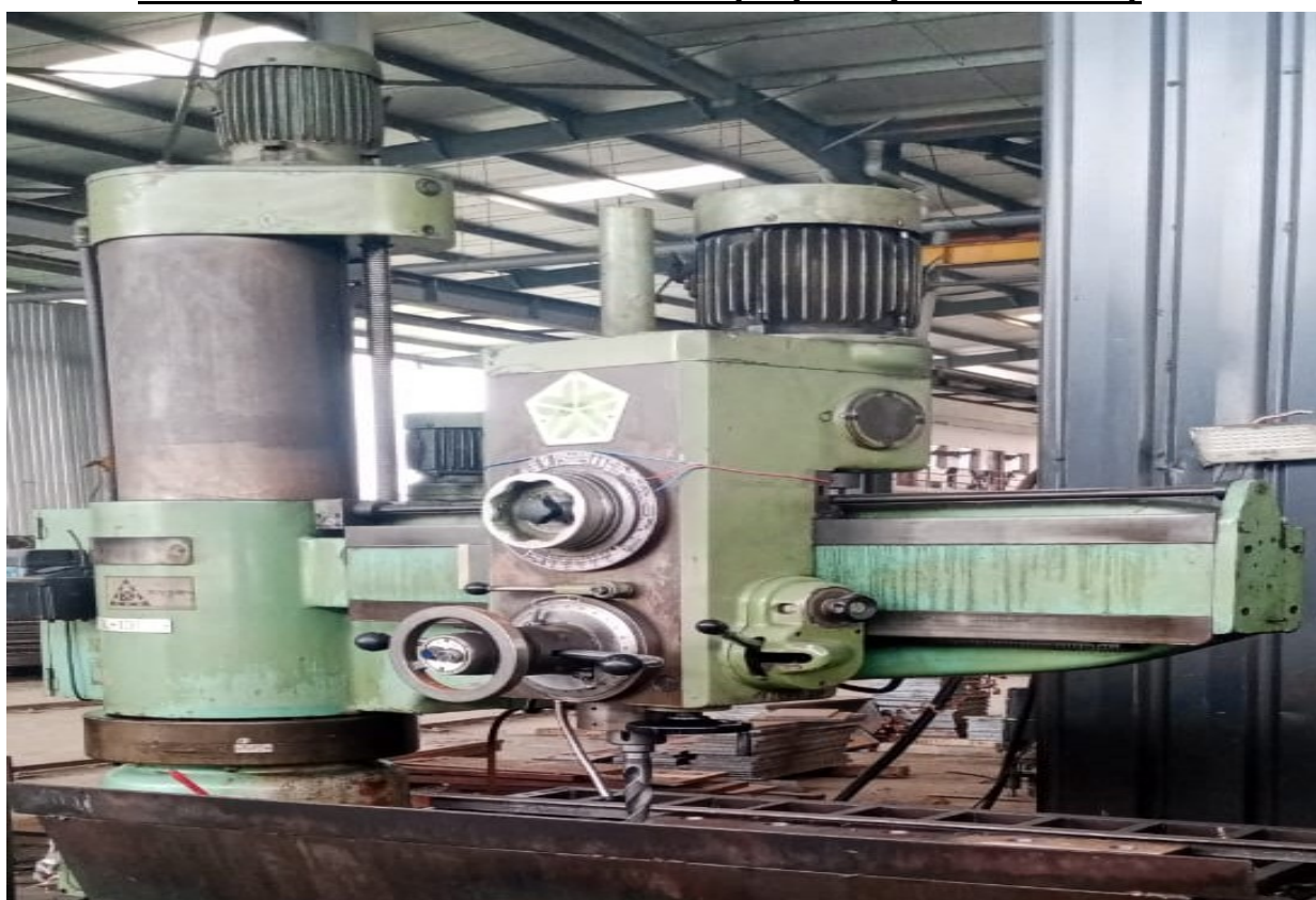
RADIAL DRILLING MACHINE-02 (Capacity-Dia-60 mm)
