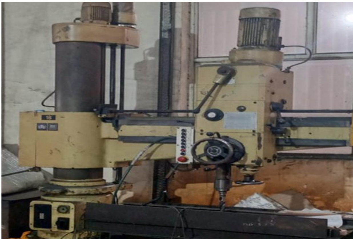
RADIAL DRILLING MACHINE-01 (Capacity-Dia-50 mm)
